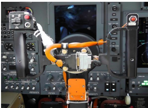
Figure 4: The data acquisition equipment to measure column forces.
